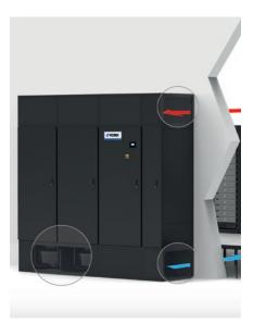
Version for installation outside the Data Centre, without raised floor, rear air supply. In this case the plinth (fixed height 550 mm) is supplied with side closure panels and rear supply air grilles. Installation of the plenum with rear reintake system is optional, if there is no ductwork.
