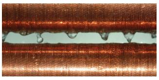
A falling-film evaporator is more efficient because refrigerant is sprayed over the tubes, offering improved heat transfer and reducing refrigerant charge by 30%.
