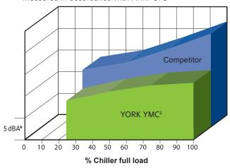
The YMC<sup>2</sup> chiller is so much quieter than competitive magnetic-bearing chillers, it sounds about half as loud. \*Note: each segment on the Y axis = 5 dBA.
