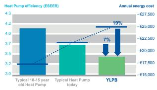
500 kW unit, 3000 operating hours, energy rate = 0.1 EUR / kWh
