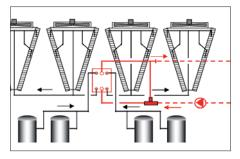
An optional heat recovery feature can be added to provide hot water to  $60^{\circ}$ C; which is useful for facility heating or hot water preheating.
